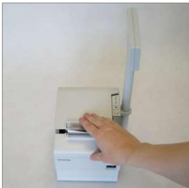
6. Release the protruding piece of paper with the serrated edge of the printer.
