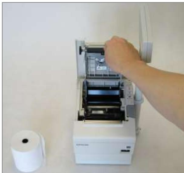
3. Insert the roller into the container so that the paper rolls off the bottom of the roll.
