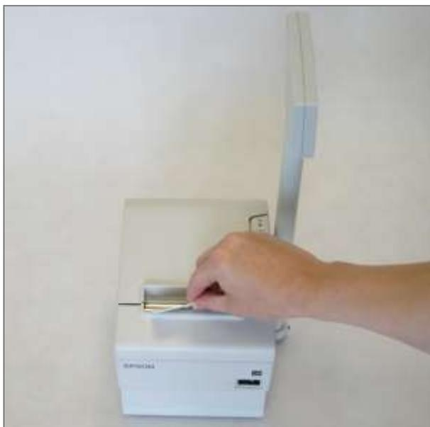
When replacing a roll for a new one, be sure to first remove the residue from the used roll of paper.
