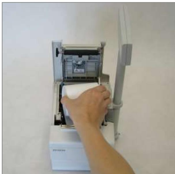
4. Before closing the cover, hold the end of the paper out of the printer.
